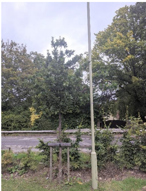
Figure 25. Poorly planned tree planting next to a lamp column
